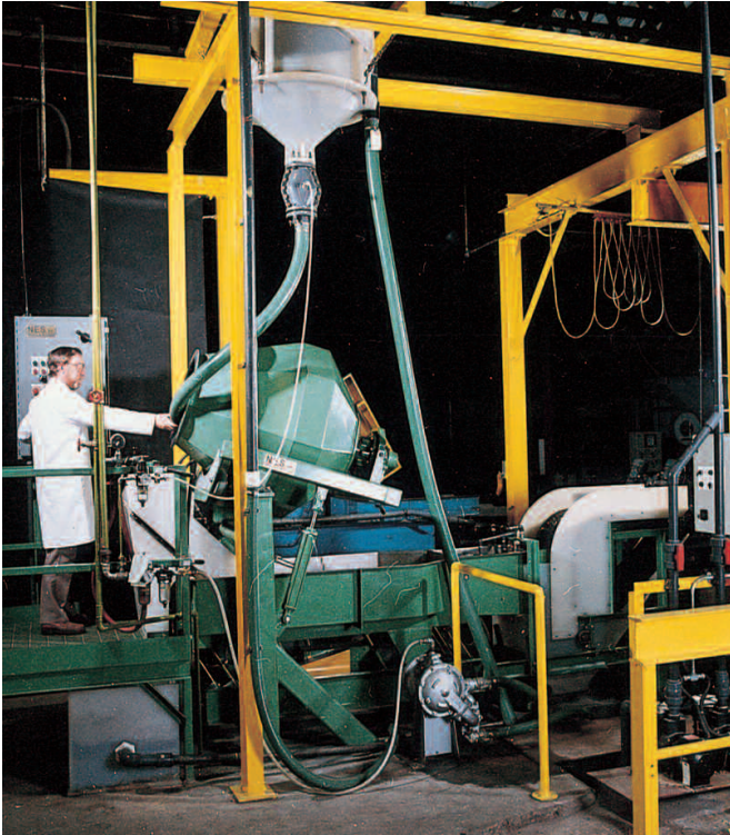
Mechanical Plating Plant
