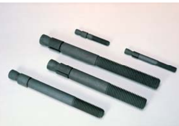
Foundation bolts demonstrating the uniformity of the coating on threaded components and the fact that finished parts can be treated prior to assembly.
